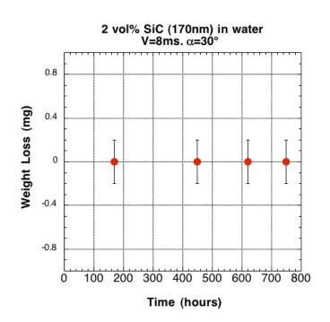
Thus far, no damage to cast aluminum of impellor of commercial automotive water pump
