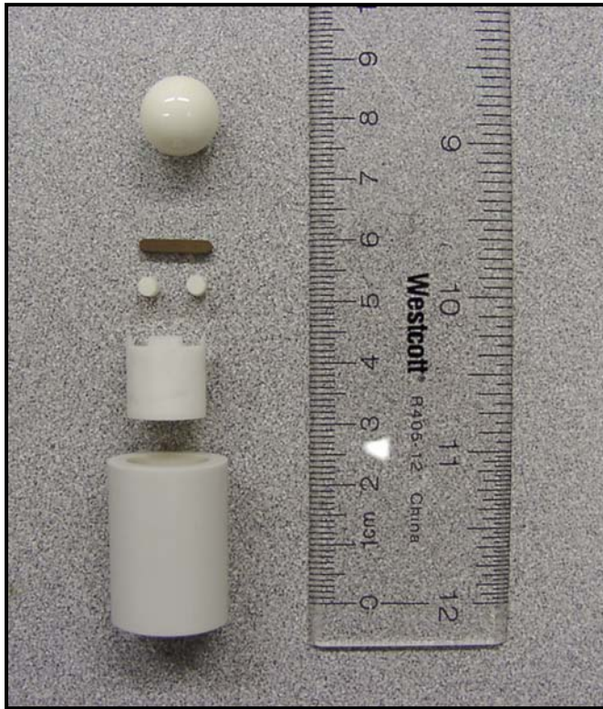
This is a “Ball on Two Rollers” 3-Point Bend Fixture
