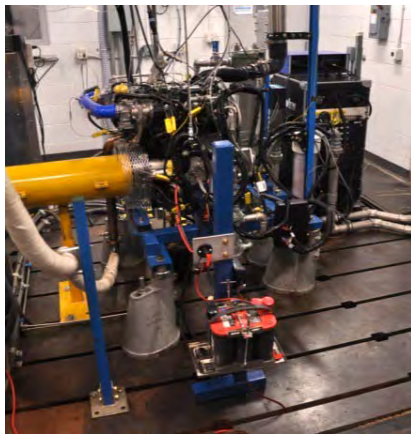
2007 MY GM 1.9-L engine installed in the test cell
