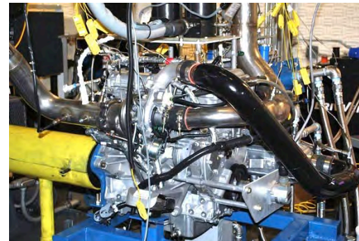
2009 MY GM 2.0-L LNF engine installed in the test cell
