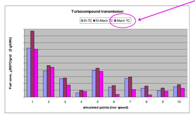
Fuel consumption results show fully mechanical transmission with fixed speed ratio to be most efficient
