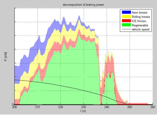
Simulation performed to investigate theoretical recovery for mild hybrid, snapshot of customer duty cycle during deceleration.
