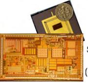
Silicon-on-Insulator Chip (chip size 10x5 mm<sup>2</sup>)
