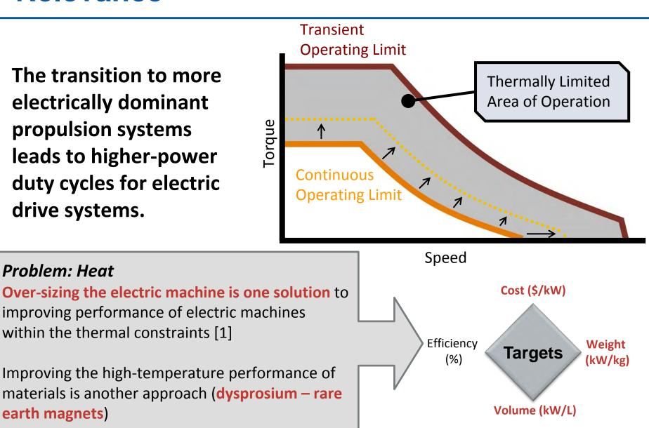
[1] Source: C. Liao, C. Chen, and T. Katcher, "Thermal Analysis for Design of High Performance Motors," ITHERM, May 1998
