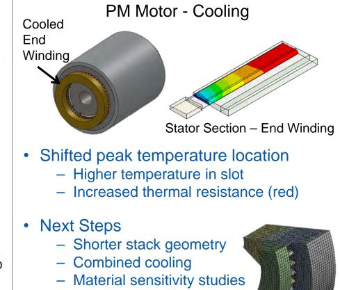
Heat spreading methods
