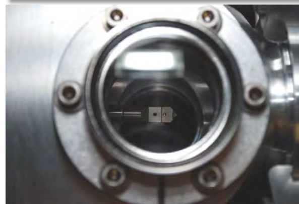
In-situ TEM holder within dry pumping station which is used to check for electrolyte leakage under vacuum before inserting into the electron microscope.
