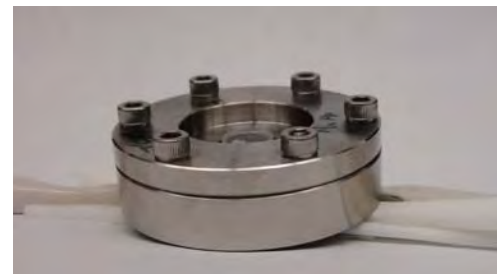
Raman Spectroscopy fixture designed to interface with CNM equipment
