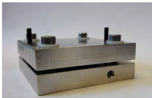
Ceramic plate electrochemical test fixture.
