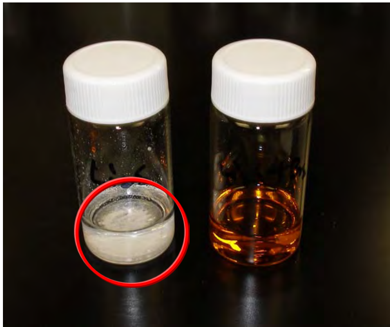
Images of \text{Li}_2\text{S} in organic solvents: Left, without \text{Br}_2 ; right, with \text{Br}_2
