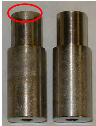
Corrosion of stainless steel parts
