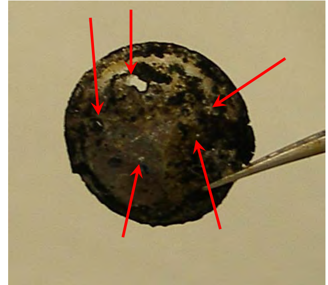
Corrosion of aluminum current collector
