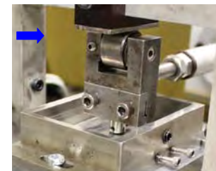
Ring-on liner configuration (similar to ASTM G-181)
