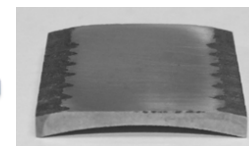
Ring-on liner configuration (similar to ASTM G-181)
