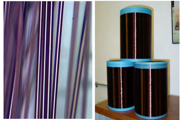
Processed Precursor Fibers from a Hardwood/Softwood Lignin Blend.
