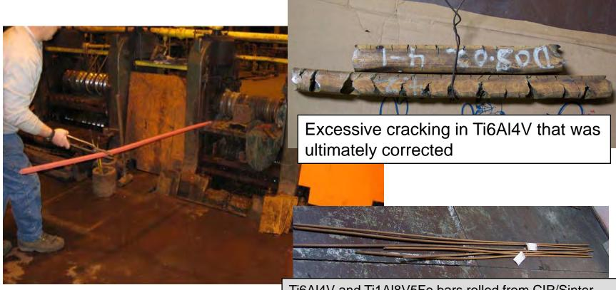
Successful rod rolling of solid state processed Ti1Al8V5Fe beta alloy
