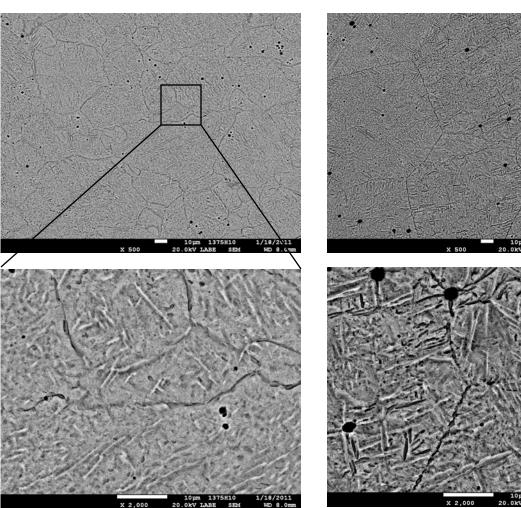
Solution Treatment 746°C for 1 hr + 4 hrs Aging at 900 F
