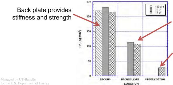
Bronze layer imparts embedability and solid lubrication during start-up and boundary lubrication
