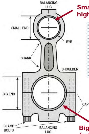
Small end bearing - piston end (oscillating, high load, low speed)
