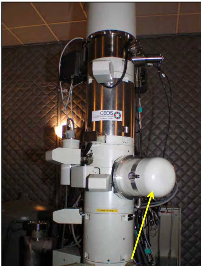
Original ACEM "clamshell" cover for specimen stage (seals holder against external disturbances such as pressure changes).
