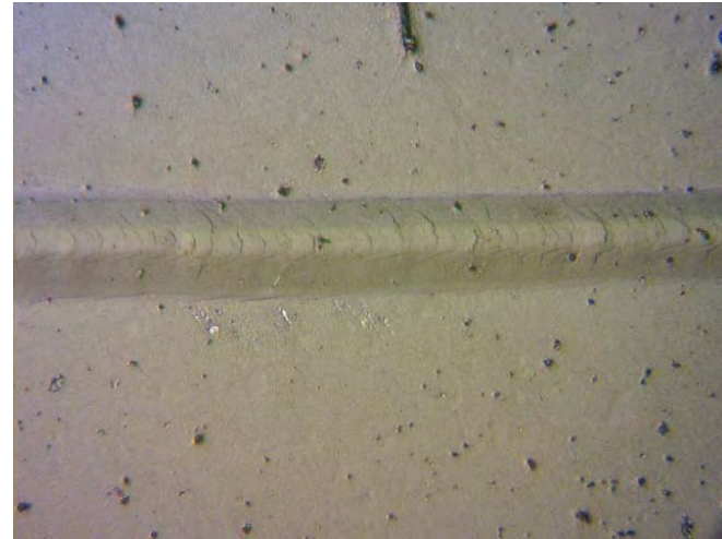
Scratch Test Track Prior to Spall
