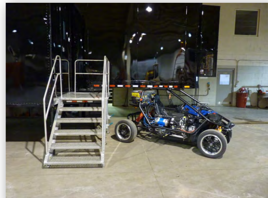
Completed Configurable Hybrid Electric Learning Vehicle which was designed and built by Senior Design students
