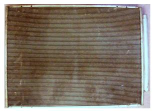
Development of Component Models Example: Condenser Model Complex heat exchanger •Multiple passes •Multi-channel tubes •Micro channels •Multiple refrigerant phases
