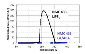
ARC profiles for NMC433 18650 cells in 1.2 M LiPF<sub>6</sub> in EC:EMC (3:7) and 1.0 M LiF/ABA in EC:EMC (3:7) at 4.3 V
