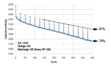
Capacity retention for 18650 cell using 3M alloy, L-20772, in 2:1 blend with graphite.
