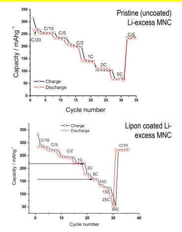
Rate Performance Comparisons at 25°C with similar electrode composition (85% active materials, 7.5 % PVDF and 7.5 % carbon (Timcal Super C65))
