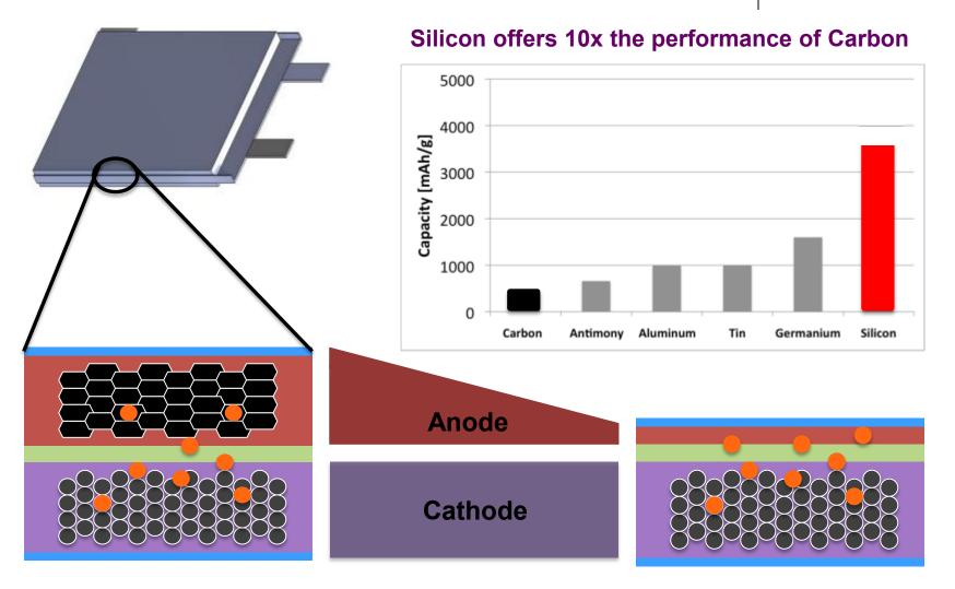
Amprius greatly improves the performance of the battery cell by shrinking the size and weight of the anode using Si
