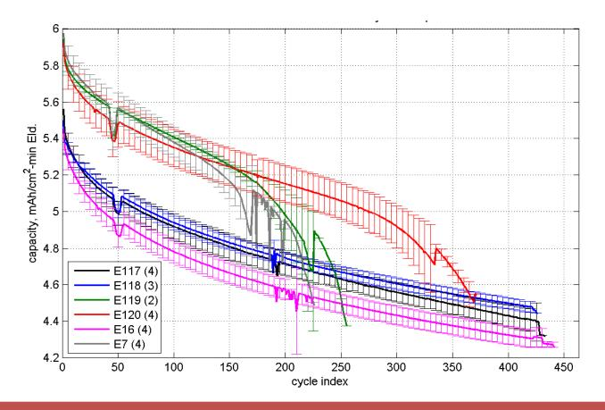
Various electrolyte formulations and additives strongly affect the cycle life in full cells
