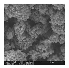
SEM image of HCMR<sup>TM</sup> Cathode cathode for high power applications)
