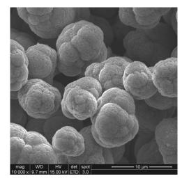
SEM image of HCMR<sup>™</sup> Cathode (dense cathode for high energy applications)
