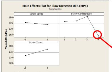
Reduction in strength observed with screw configuration #4 is due to inadequate fiber dispersion and wet out
