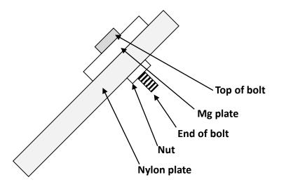
Side of substrate holder (inclined 45 degrees)
