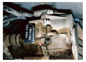
Transfer case exhibiting perforation and oil leak without effective isolation
