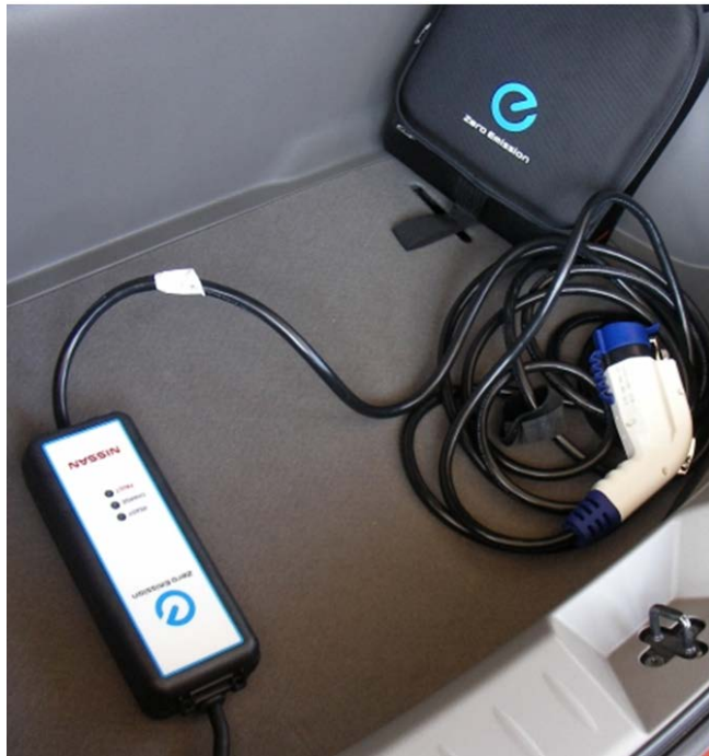
Nissan Leaf On-board Convenience Charger (Panasonic 120v/15A input)
