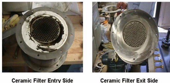
Figure 2. Entry and Exit Sides of the Filter Cartridge After a 1.2 Liter Diesel Engine Filtration Cycle
