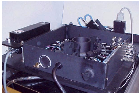
Figure 1. Diesel Particle Scatterometer calculations using a Levenburg-Marquardt optimization program. The result is plotted as a size distribution and refractive and absorptive optical properties of the particles. The absorptive component of the index of refraction gives a measure of the graphic carbon content of the exhaust particles. An important advantage of the instrument is the rapid response time; it has been tested at greater than 1 Hz data acquisition rate. This speed allows for the measurement of engine transients and even cylinder-to-cylinder to variations.
