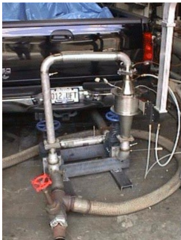
Figure 3. Test Apparatus on the Exhaust of a 7.3 Liter Light-Duty Diesel Truck
