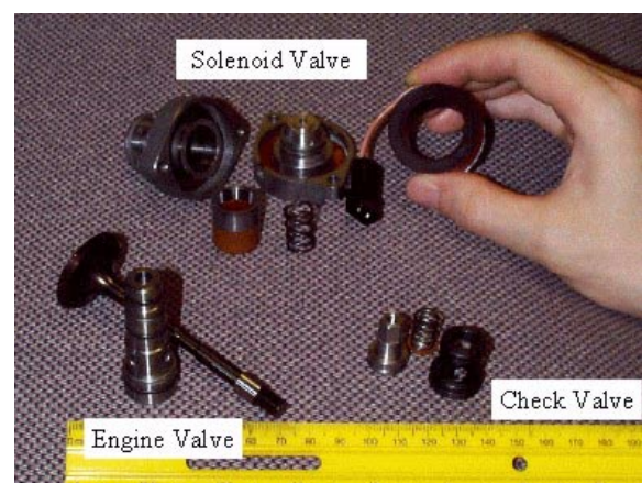
Figure 1. Electrohydraulic Camless Valvetrain Components
