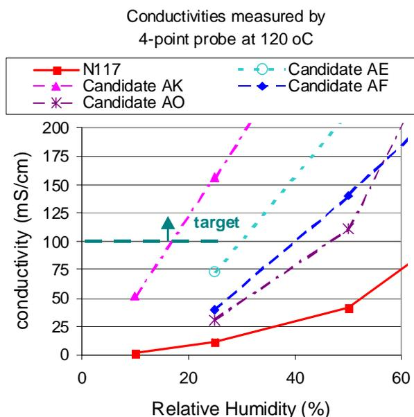
Hydrogen ion conductivity at 120°C of newly-synthesized polymer electrolyte materials as a function of relative humidity. Baseline material is N17.
