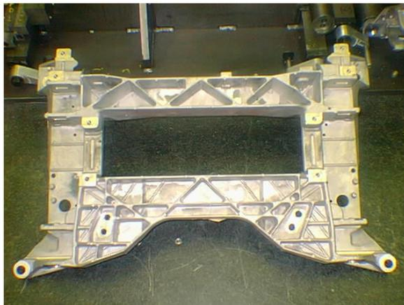
**Prototype Magnesium Front Engine Cradle Casting**
