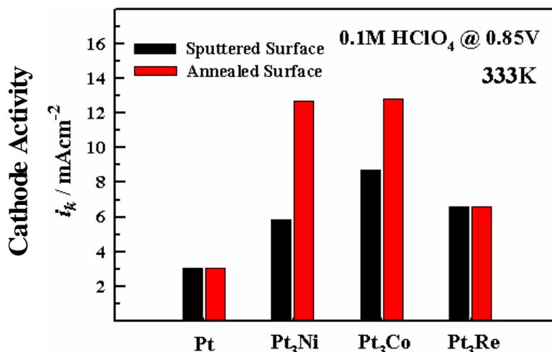
Pt-alloy systems with (annealed) and without (sputtered) all-Pt surface “skin” layers, compared to pure Pt
