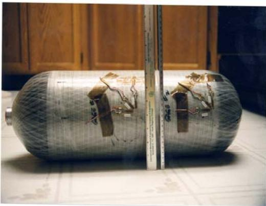
Test pressure vessel was instrumented with strain gages to measure the effect of stresses.
