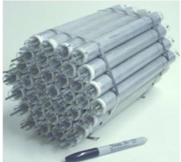
Figure 5. Plasma Reactor for 60-kW Diesel Engine
