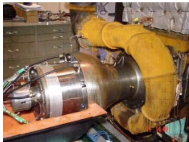
Figure 4. Electric Turbocharger Installed on Test Stand
