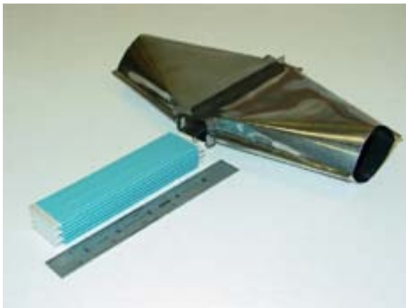
Figure 6. Stainless steel sheet metal NTP reactor housing and ceramic dielectric stack.
