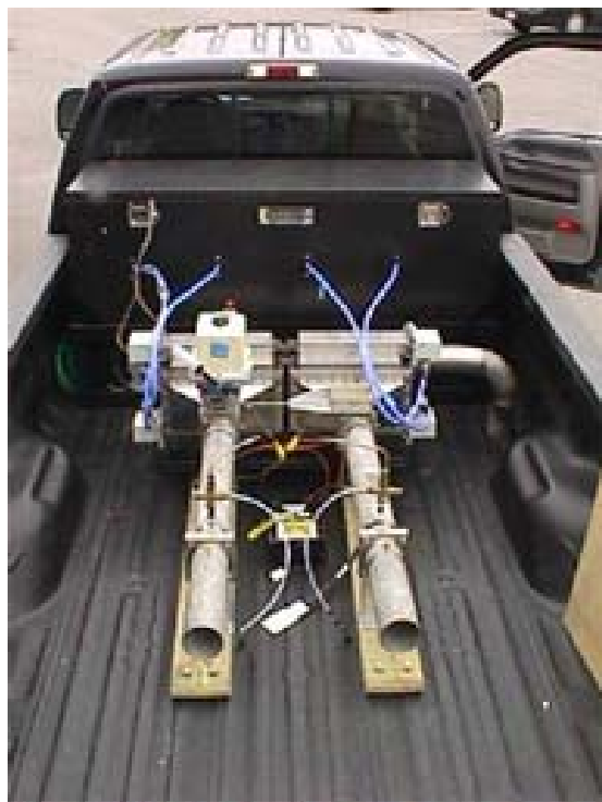
Figure 5. Microwave-regenerated pleated cartridge DPF installed on a Ford 7.3-L truck for testing.
