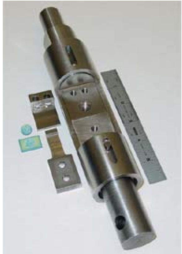
Figure 3. Shear test fixture assembly used to measure the shear strength of the sealing glass joint.
