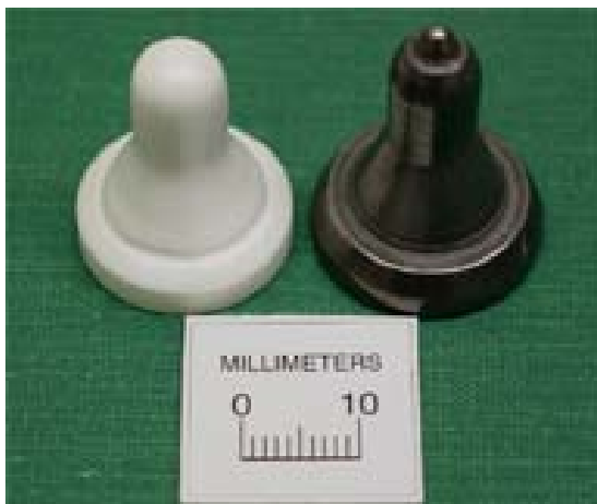
Figure 4. Gelcast and sintered ZrO_2 fuel injector nozzle shape (left) containing an array of eight holes in the tip. A steel nozzle is shown at right.
