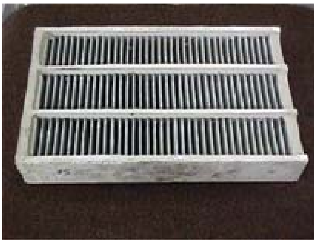
Figure 1. The new design of the ceramic fiber pleated filter cartridge.
