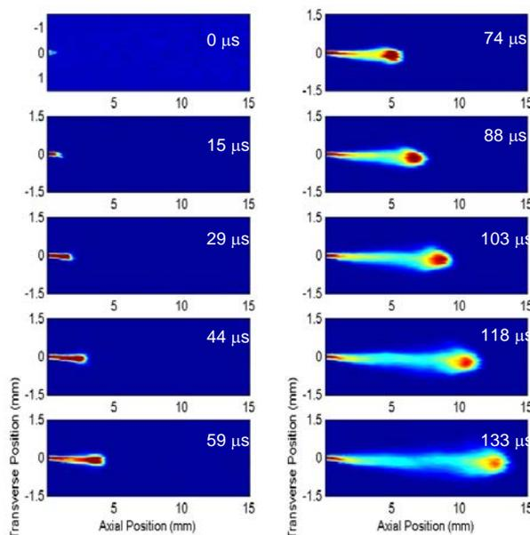
**Spray evolution in a 5-bar nitrogen environment with 500-bar injection pressure**
