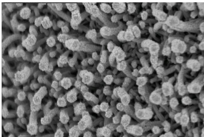
**Polymer whiskers coated with a continuous thin layer of platinum**
