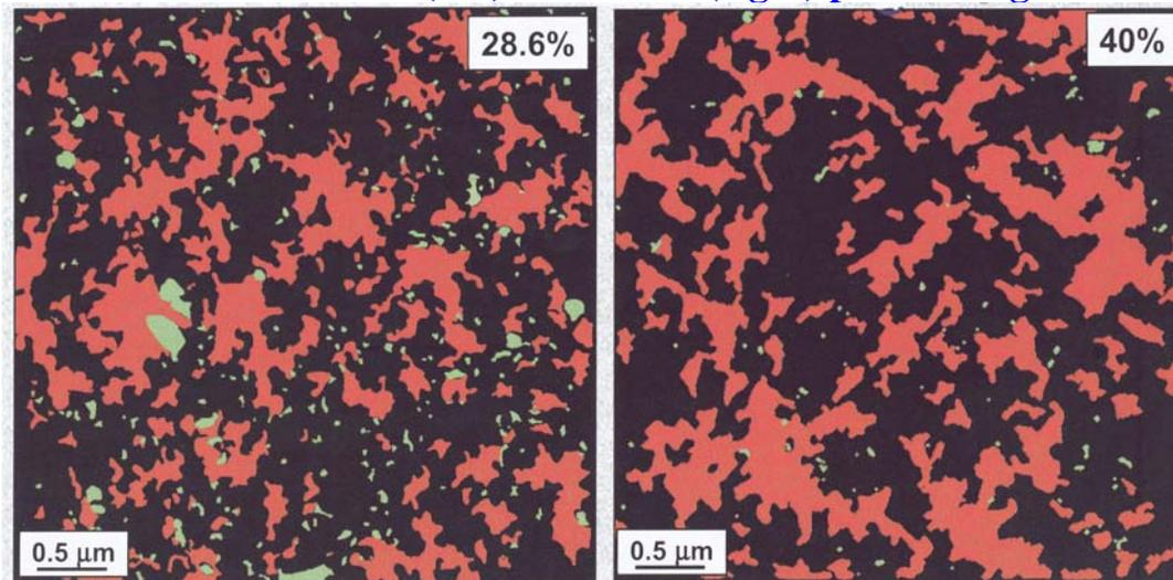
(color code: platinized-carbon, ionomer, open pores)
