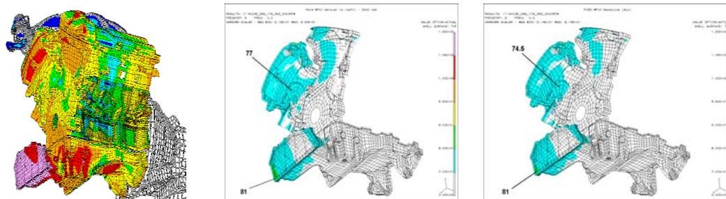
**Acoustic Analysis of Mg-Intensive Engine (overall and Mg vs. Al redesign)**
