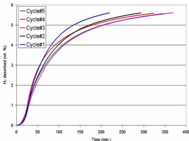
Hydrogen generation over time showing 5.5 wt% capacity
