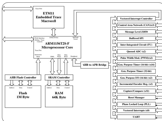
**High-Level Functional Block Diagram of SoC Motor Controller**
