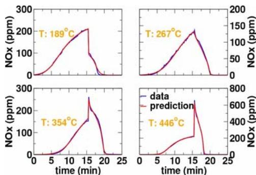
NO<sub>x</sub> concentration after adsorber for four temperatures (adsorption 0-15 minutes, desorption 15-25 minutes). The red curves indicate the predicted response; the blue curves show the experimental data.
