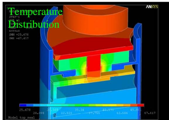
**Analysis of Current Density and Temperature Distribution in Saft Li-Ion Cell**
