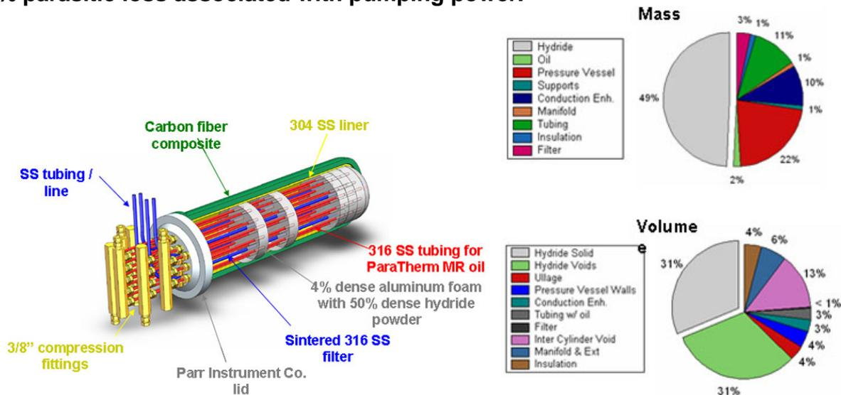
1-kg hydrogen prototype cutaway and mass and volume distribution for a 5-kg system using 1-kg first generation prototype modules.
