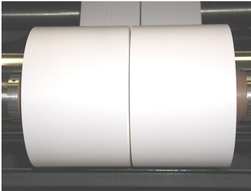
**On-line slitting of 1700 m Teklon<sup>®</sup> rolls onto 3" ID cardboard cores**
