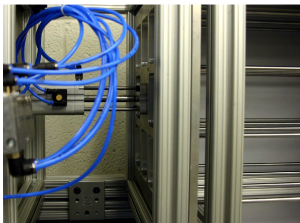
Figure 2. Detail of environmental chamber showing pneumatic actuator and frame with sixteen 6.5-mm diameter rods.
