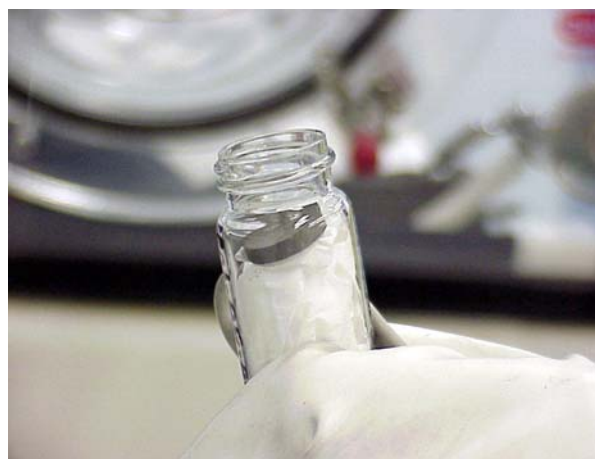
Figure 3. Near-final-shape compact with an L/D ratio of 0.21 (L = 15.9 mm).
