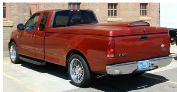
Figure 4. Baseline performance tested 100% hydrogen, 32-valve, 5.4 liter internal combustion engine pickup.
