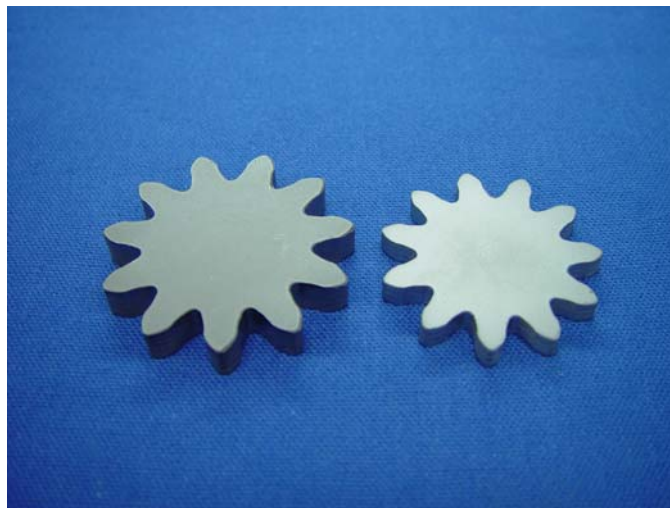
Examples of powder-metallurgy titanium oil-pump gears made from low-cost titanium powder at PNNL
