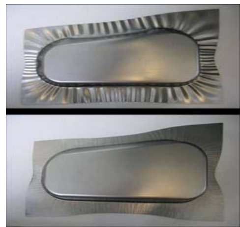
Figure 2: Steel Pan drawn without (upper photo) and with closed loop control (lower photo)
