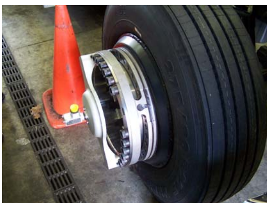
Figure 1. Wheel Force Transducer Loaned to Support HTDC Pilot Testing, from Dana Corporation
