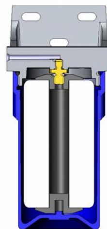
Figure 2. Engineering View of a RGS Oil Bypass Filter
