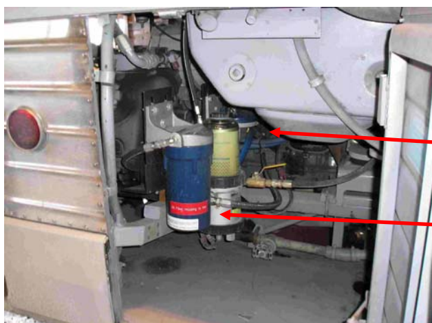
Figure 4. RGS Oil Bypass Filter Installed on an INL Bus
