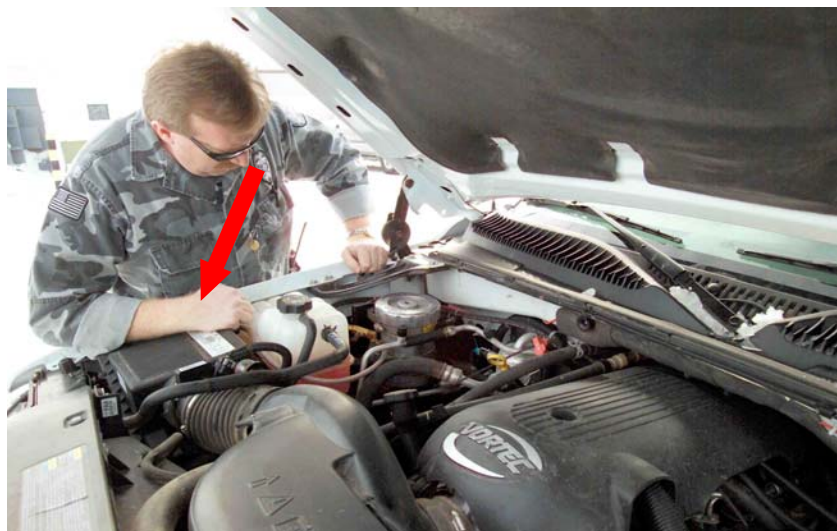
Figure 8. INL Personnel Viewing the Location of the Oil Bypass Filter Installation in the Engine Compartment of an INL Chevrolet Tahoe
