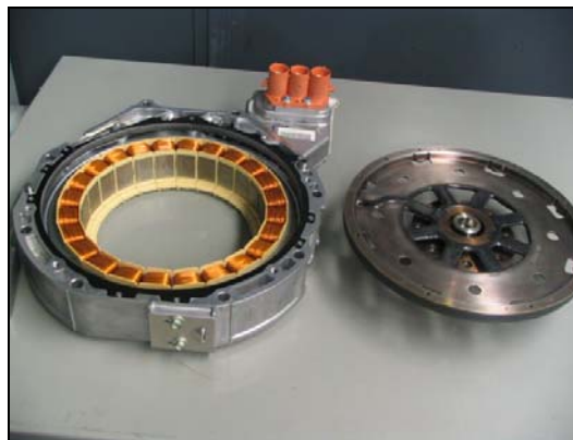
Figure 1. Digital Telemetry Torque Sensor Antenna (left) and Sensing Flexplate (right)
