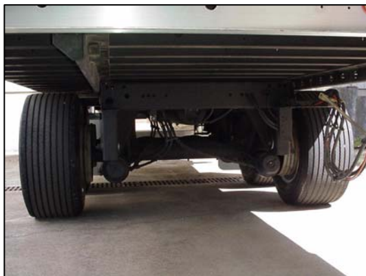
Figure 3. NGSBWTs Mounted on the Dana Trailer Used in the HTDC Pilot Test
