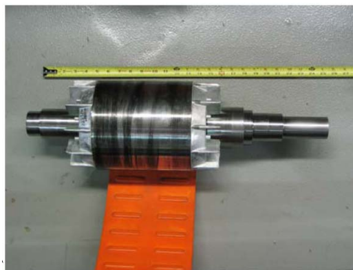
Figure 11. New Double-Ended Shaft Pressed in the NEMA Machine Rotor
