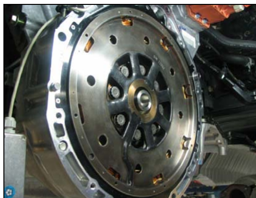
Figure 2. Torque Sensor Installed in Flexplate Location
