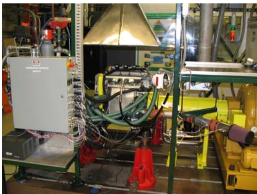
Figure 2. Hydrogen Engine and Test Cell
