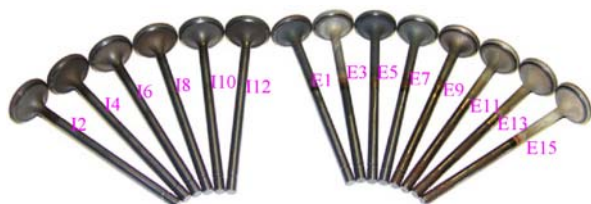
Figure 6. Photograph of 100-h engine-tested \text{Si}_3\text{N}_4 and TiAl valves.
