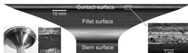
Figure 2. Laser-scatter scan image of head surface of TiAl valve #1 after 20-h cyclic-impact rig test.
