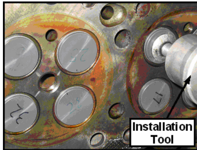
Figure 3 \text{Si}_3\text{N}_4 valve under compression from an installation tool
