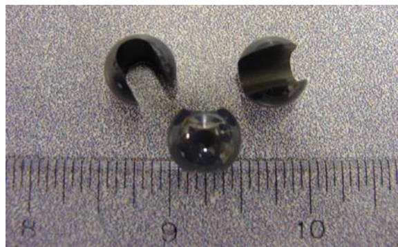
Figure 5. Machined \text{Si}_3\text{N}_4 C-sphere flexure strength specimens.
