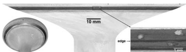
Figure 10. Laser-scatter scan image (in log-intensity scale) of TiAl valve #8 (at E15 in engine) after 100-h engine test.
