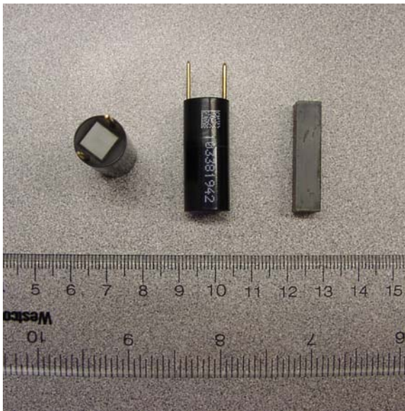
Figure 1. Examples of piezo-stack actuators. Left is a top view, middle is a side view, and right is a stack removed from the protective covering.
