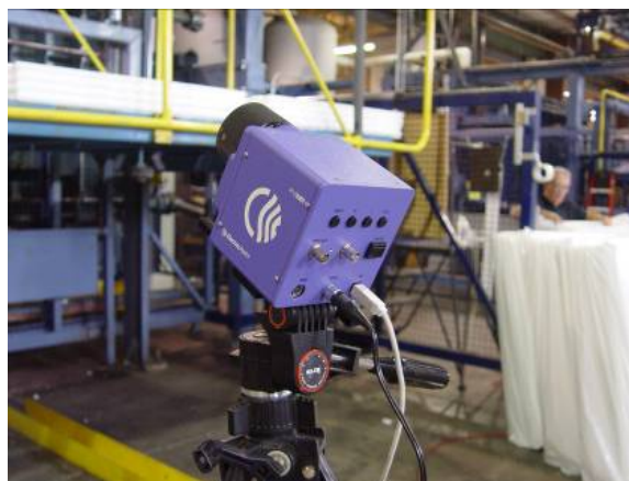
Figure 3. Infrared camera installation at a molding operation.
