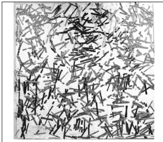
Figure 7. Composite hybrid preform with 3% carbon fiber chop.
