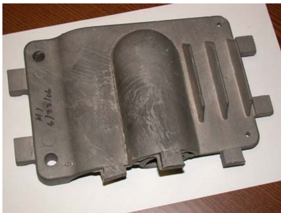
Figure 4. A geometrically perfect Mg alloy lost foam casting made using the Hitchiner process.
