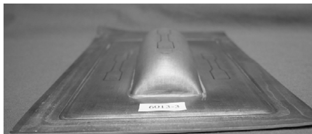
Figure 7. Typical formed 6xxx alloy tray representing 100% elongation (0.7 strain).
