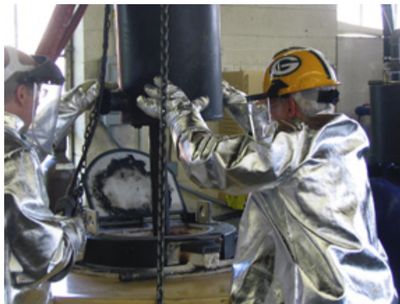
Figure 1. The Hitchiner casting system is being tested by TTU and ORNL researchers for lost foam casting of Mg alloys.
