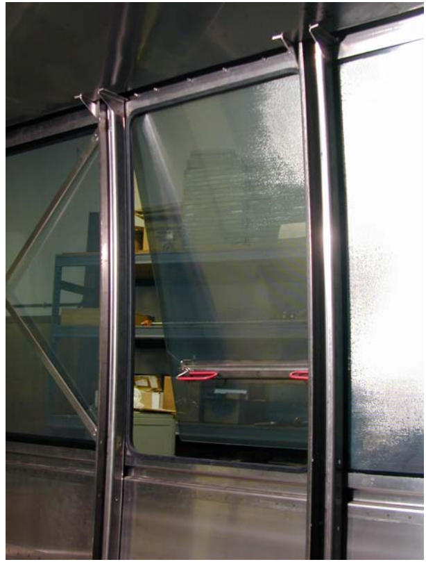
Figure 3. Emergency exit window.
