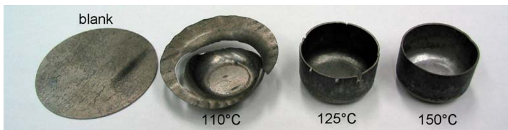
Figure 3. Effect of temperature on drawing operations.
