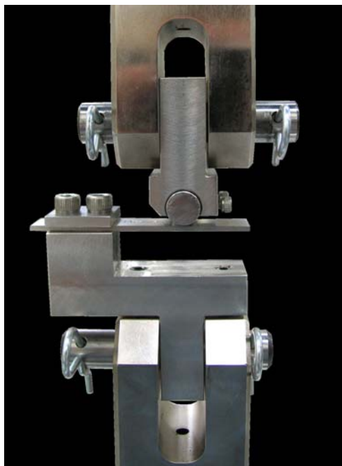
Figure 1. This cylinder-on-flat fretting configuration was designed to fit existing fatigue testing frames. The cylinder specimen diameter is 9.53 mm.
