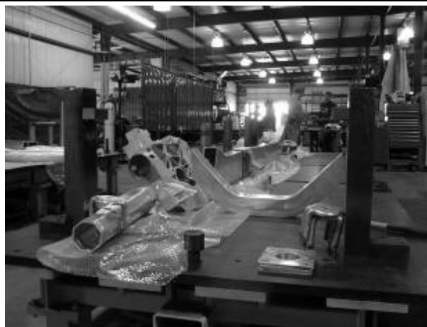
Figure 1. NGF components and assembly fixture before final assembly.
