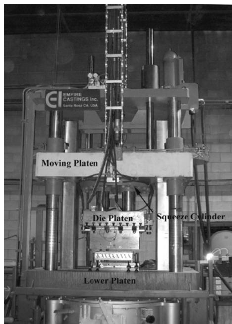
Figure 1. ASC machine installed at Eck Industries.
