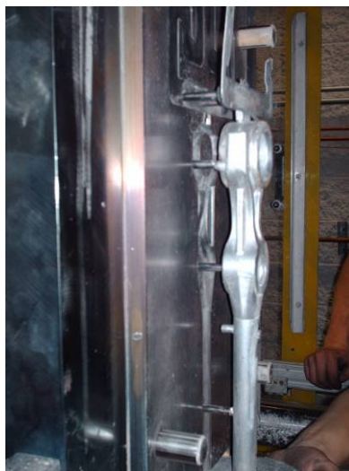
Figure 15. Initial magnesium connecting rod casting in die.
