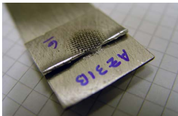
Figure 7. Base metal failure during peel test AZ31B ultrasonic weld.
