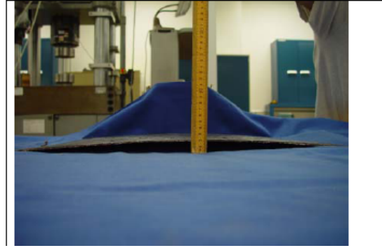
Figure 3. Warpage of the hybrid panel after molding.
