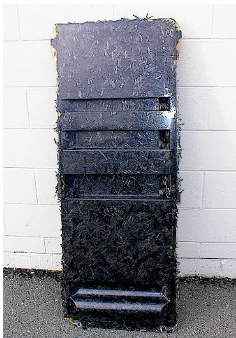
Figure 18. Molded preform indicating discontinuous fiber surface.
