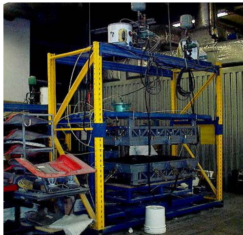
Figure 22. Mold cell for test tool setup for large part molding.
