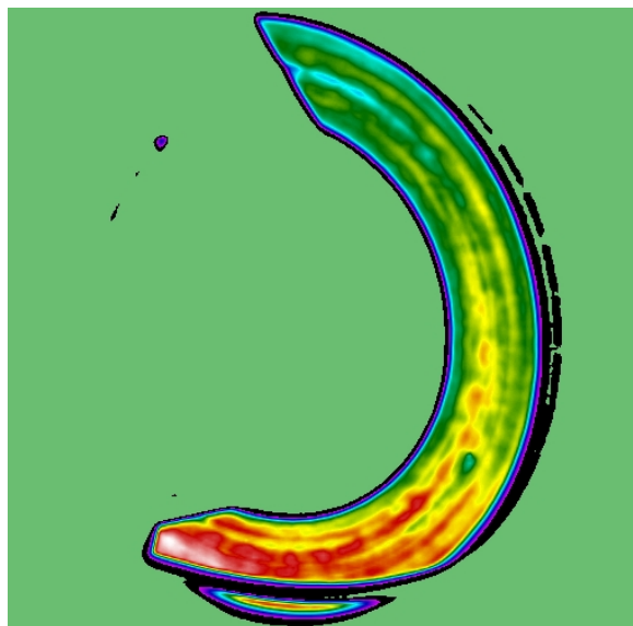
Figure 4. Infrared (IR) thermal image of the Ti rotor during the sixth snub stop. Red represents a temperature of about 1600°F and dark blue about 1200°F. Dashed dark streaks at the right edge of the disk are cooling vents.
