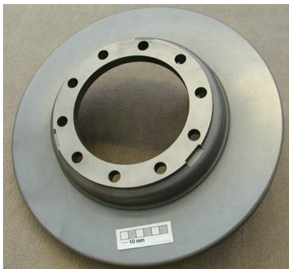
Figure 1. One of the first four full-scale, thermally sprayed titanium truck brake rotors to be produced. It was prepared for this project by Red Devil Brakes, Inc., of Pennsylvania.
