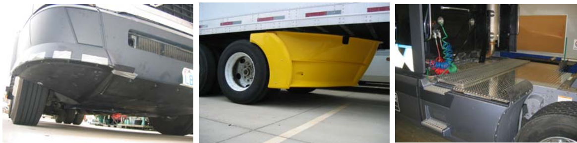
Figure 9. Volvo smooth tractor underside concept (left), trailer bogie deflector (center), and deck enclosure (right)
