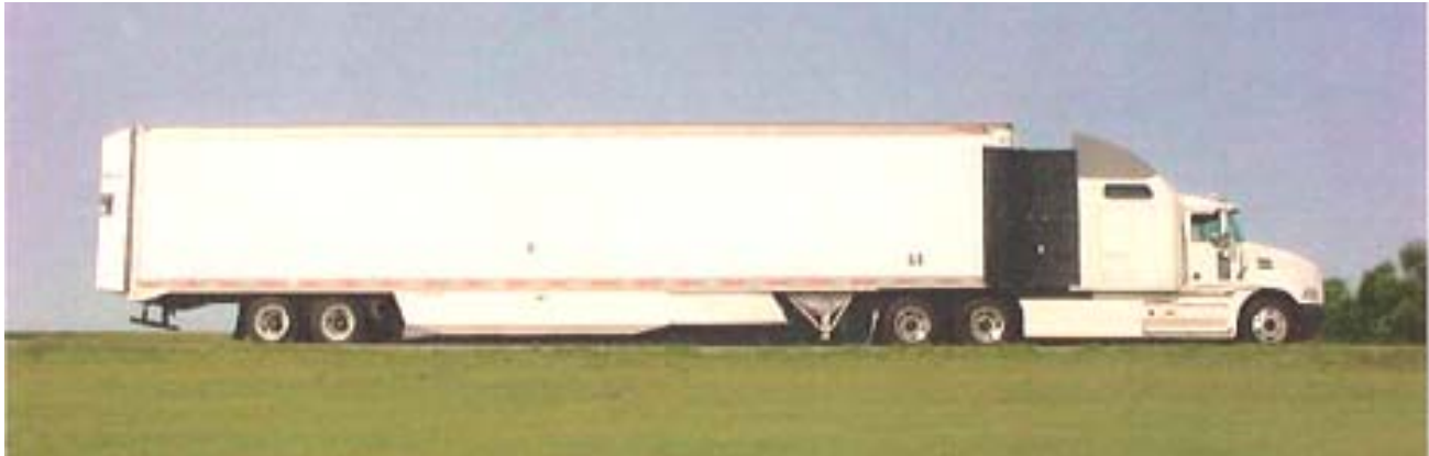
Figure 7. Mack tractor-trailer combination including side enclosures, trailer skirts, and 2 foot boat tail
