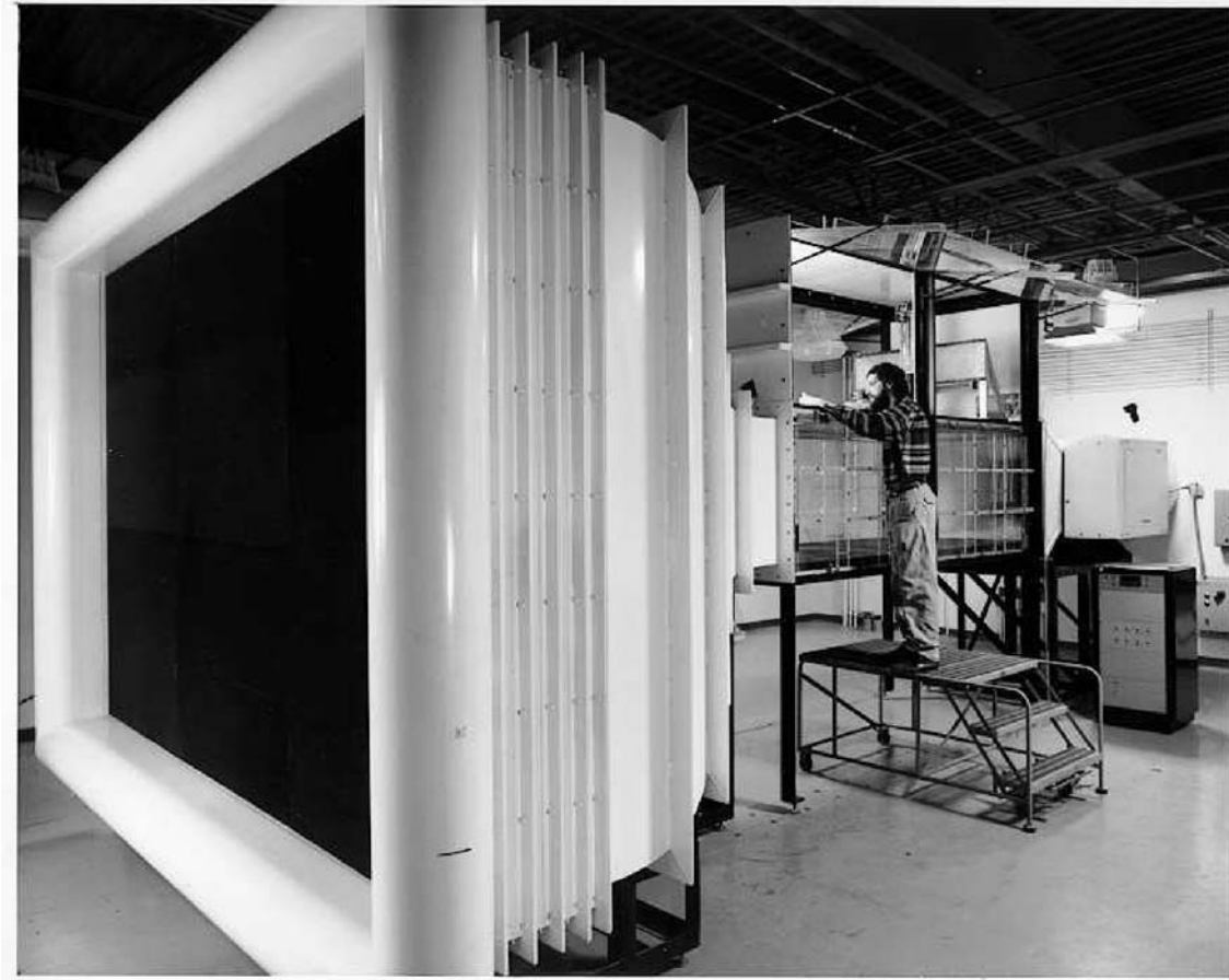
Figure 1. NASA Ames 48- by 32-Inch Subsonic Wind Tunnel (Inlet at left, plenum chamber above with doors open, test section below)
