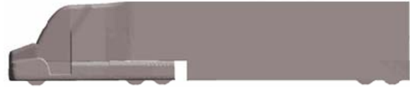
Figure 5. “GTS” configuration of the GCM, with full gap fairing and trailer belly box
