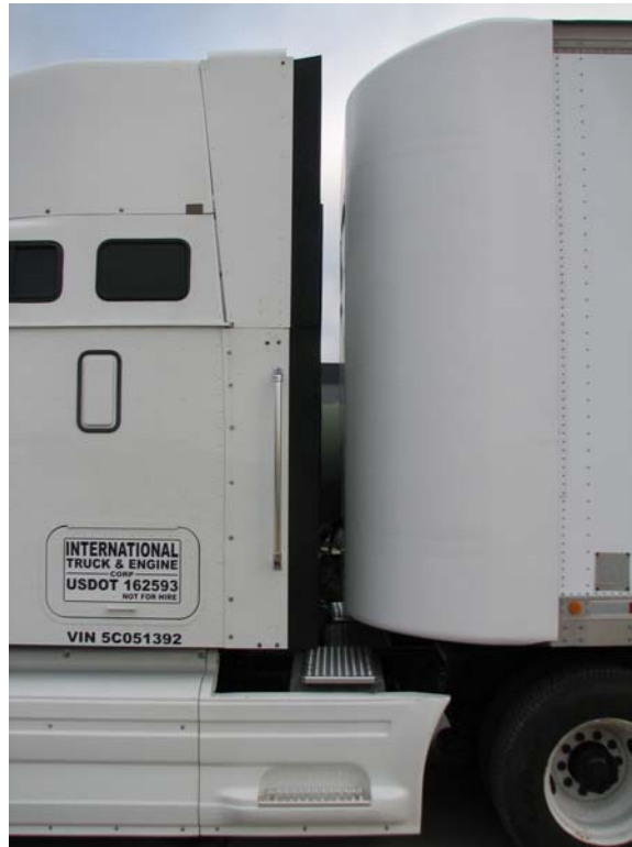
Figure 5. Trailer forebody device developed by International
