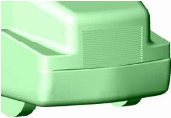
Figure 10. Modified GCM geometry with open grille and flow-through radiator
