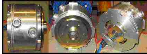
Figure 3. 20kW cooling fan motor
