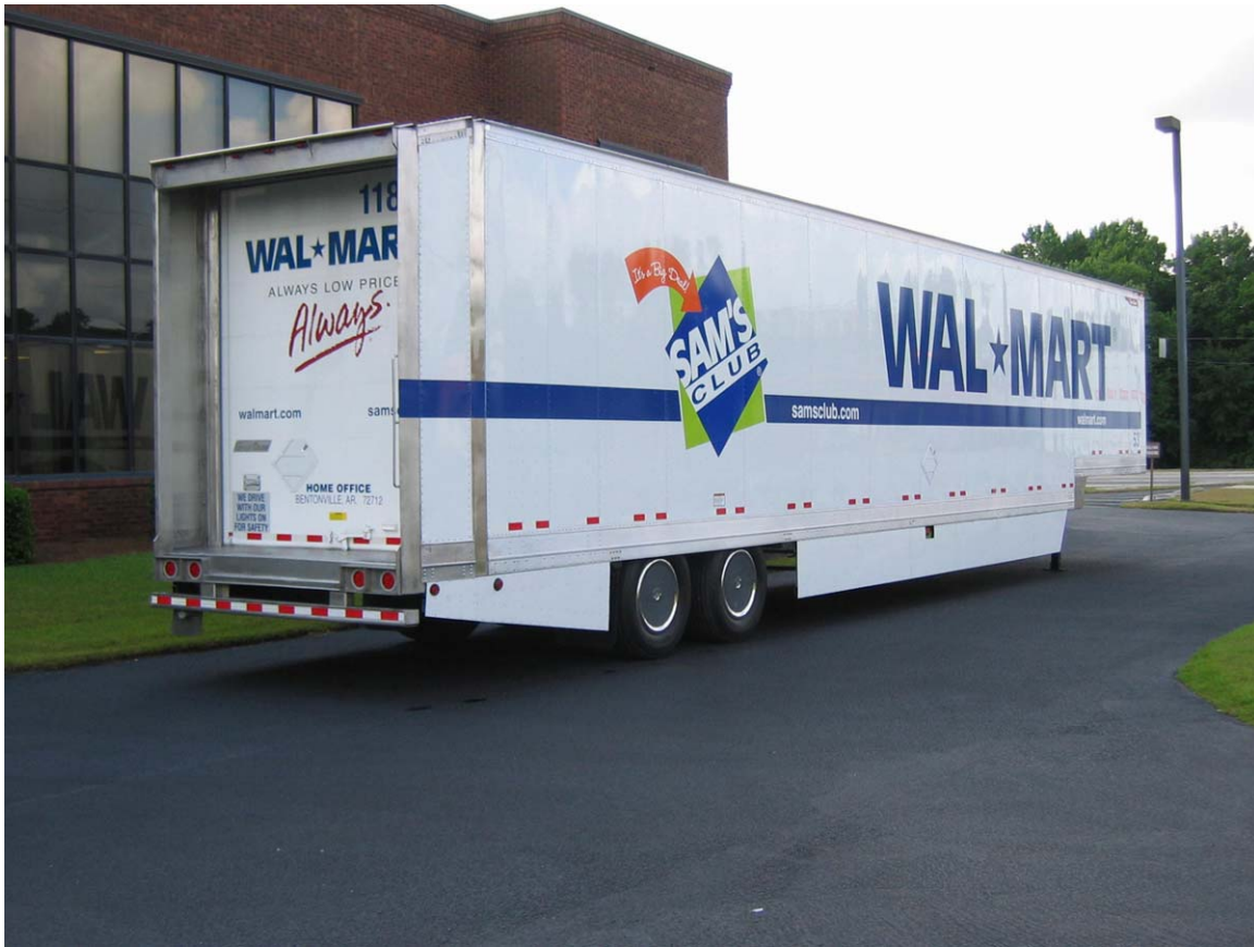
Figure 4. Experimental aerodynamic trailer developed in conjunction with Great Dane and Wal-Mart
