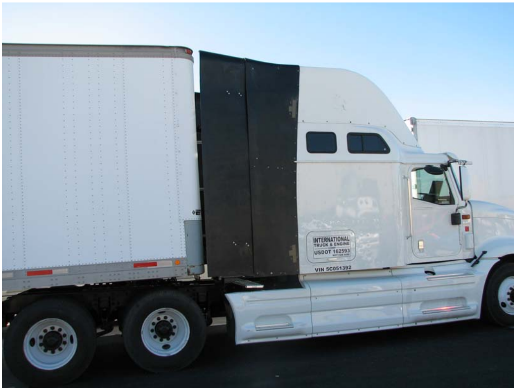
Figure 6. Variable length side extenders developed by International, in deployed position
