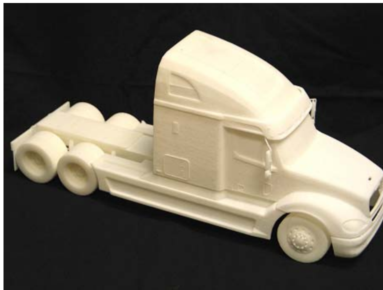
Figure 10. Wind tunnel model (1:20 scale) for testing the tractor and trailer base bleeding concepts at NASA Ames in FY07
