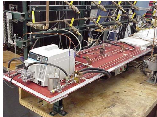
Figure 2. Picture of nanofluid heat transfer test facility
