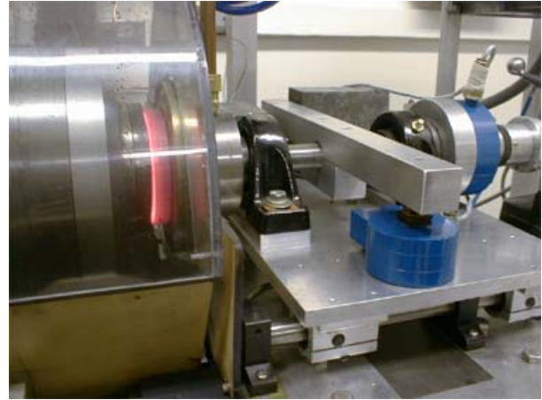
Figure 8. Subscale wear/durability tester at Rockwell Scientific
