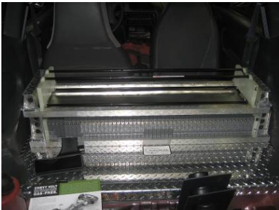
Figure 10. 5kWh NiMh Battery
