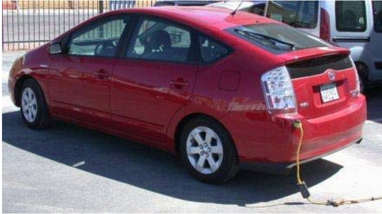
Figure 4. Prius converted to a PHEV by Hymotion. Note the 110 volt connector cord in the bottom left of the vehicle bumper.
