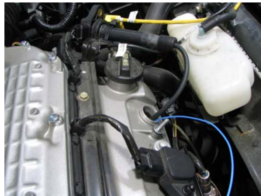
Figure 6. Honda Accord HEV with Indicated Torque Sensor (pressure transducers are inside the spark plug)
