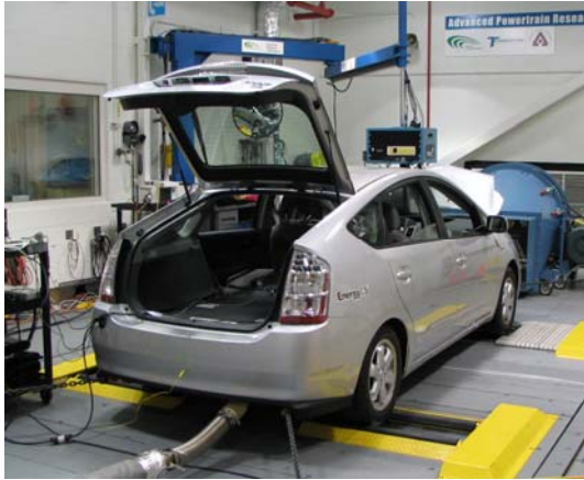
Figure 3. EnergyCS Prius Tested in Cooperation with INL and AVTA
