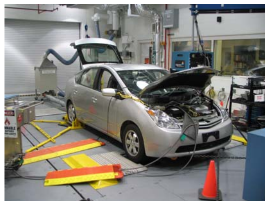
Figure 6. HybridsPlus Prius with 9-kWh Pack
