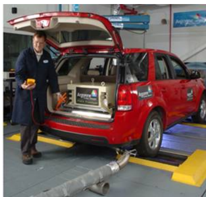
Figure 1. Argonne's Saturn Vue Installed on 4WD Chassis Dynamometer
