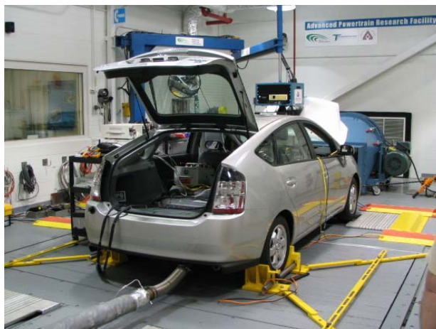
Figure 1. Hymotion Prius with Kokum Li-Ion and Level 2 Instrumentation
