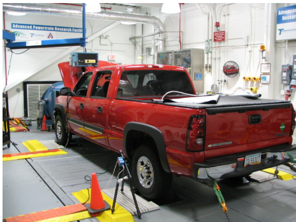
Figure 1. Hydrogen-Converted Truck Being Tested at APRF
