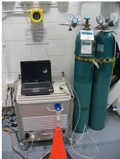
Figure 2. Analyzer to Measure Water Content in Exhaust Stream
