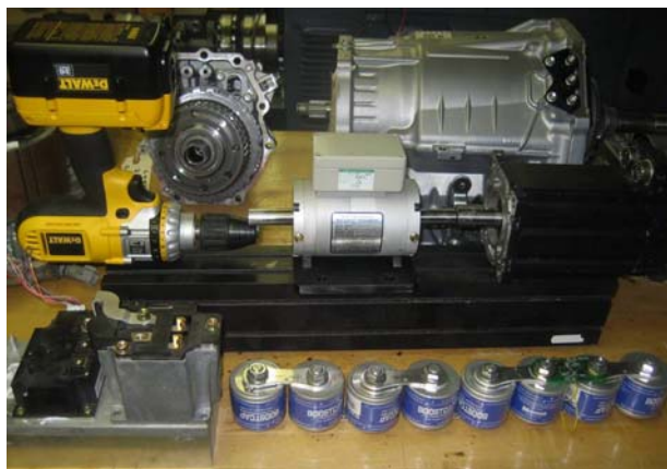
Figure 14. A Miniature HIL Set-up for Proof of Concept and Control Development
