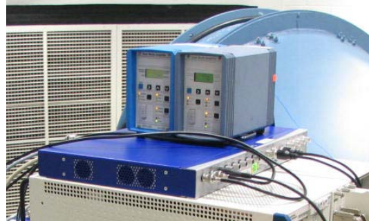
Figure 5. Indicated Torque System for Measuring In-Cylinder pressure (pressure transducers are placed inside custom spark plugs)
