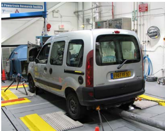
Figure 4. Renault Kangoo – Series PHEV Tested in Cooperation with INL and AVTA
