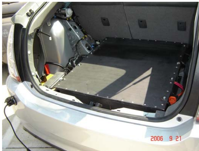
Figure 3. Lithium ion battery pack placement in the EnergyCS conversion of a Toyota Prius. The pack is in the black box. Note the 110 volt connector cord in the bottom left of the picture.
