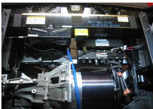
Figure 6. Installation of the UQM Electric Motor to the Rear Transaxle Assembly
