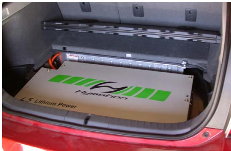
Figure 5. A123 lithium ion battery pack placement in the Hymotion conversion of a Toyota Prius. The pack sits between the rear of the vehicle and the original Prius battery which is retained and used (The Prius battery is to the right of the bright orange cables and only the upper rear side is visible as bright metal).
