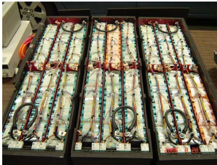
Figure 2. Lithium ion battery pack used in EnergyCS conversion of a Toyota Prius.
