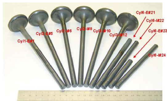
Figure 7. Photograph of \text{Si}_3\text{N}_4 engine valves at end of engine duration test.
