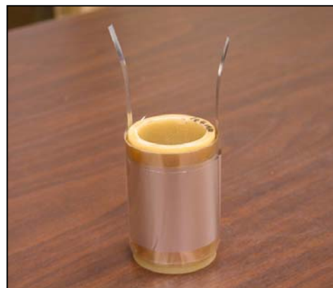
Figure 1. A 0.2- \mu F wound capacitor. Photo provided by Sandia National Laboratory.
