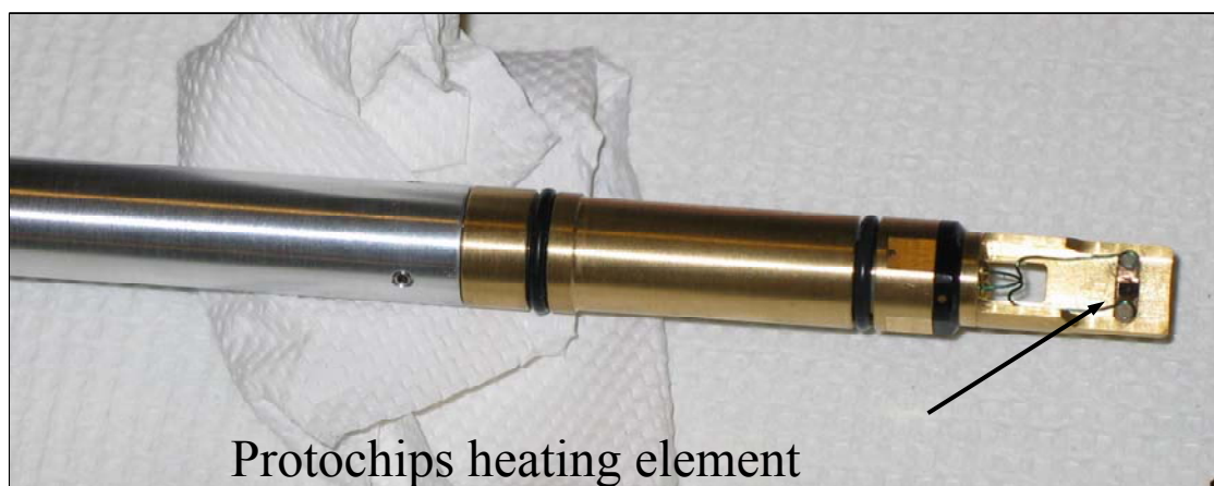
Fig. 8. New ACEM specimen heater rod, fabricated to accommodate Protochips heater chip, as indicated.
