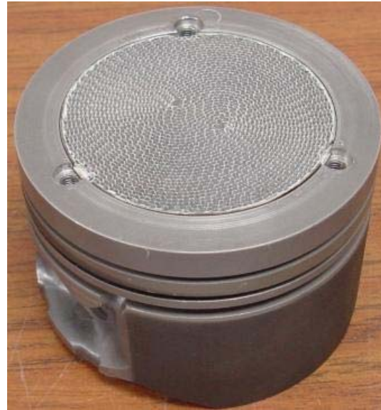
Figure 3. HCCI engine piston showing HCCI catalyst mounted in specially machined piston bowl.
