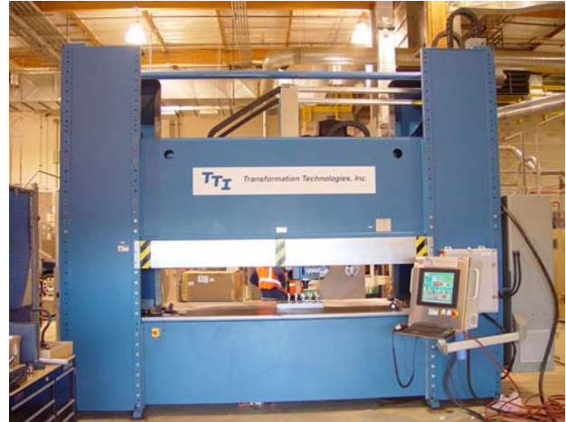
Figure 4 - Friction Stir machine at PNNL. This machine has an 8 ft. horizontal by ~ 5 ft. vertical working envelope, and a 30,000 lb Z force and 8000 lb X Force capability, while maintaining a 0.0002" spindle run out so that ceramic tooling can be used.
