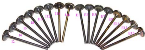
Figure 1. Photograph of 500-h engine-tested \text{Si}_3\text{N}_4 and TiAl valves.
