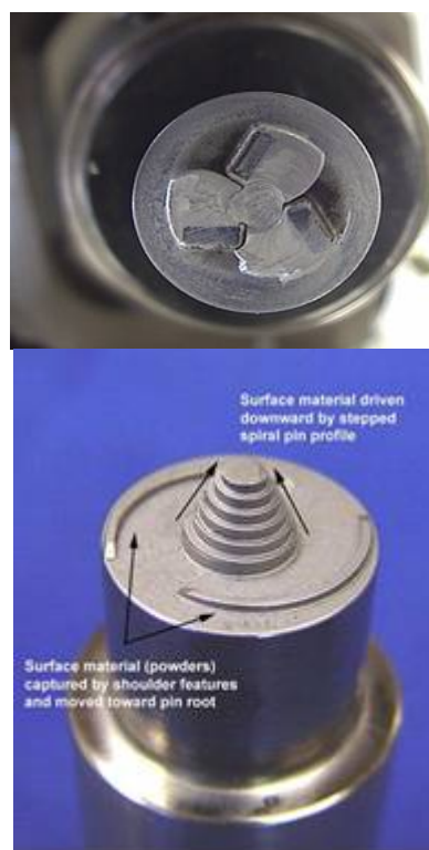
Figure 2 - Tool design is a critical component of successful FSP
