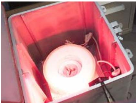
Figure 8: Sample furnace at 1000°C for the resonant ultrasound spectroscopy of diesel particulate filters.
