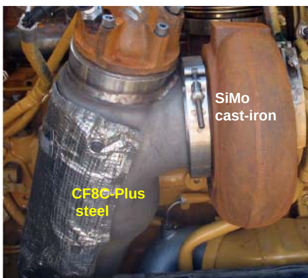
Caterpillar Regeneration System (CRS) Housing
