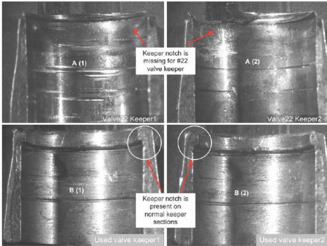
Figure 11. (A) Failed valve keeper from Cylinder #6. (B) Engine-tested valve keeper with unworn keeper latch.
