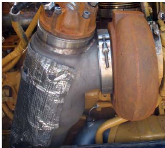
Figure 7. The first commercial application of CF8C-Plus is the Caterpillar Regeneration System (CRS) housing, which was included on all on-highway truck diesel engines after January 2007. This combustor ignites exhaust gas and injected diesel fuel to clean diesel particulate filters, and must withstand high temperatures and rapid thermal cycling.
