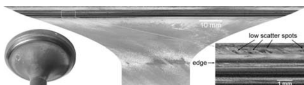
Figure 5. Laser-scatter scan image of TiAl exhaust valve E9 after 500-h engine test.
