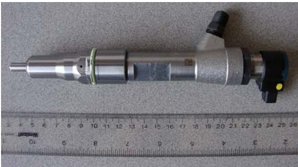
Figure 1. Piezo-actuated fuel injector used in Ford 6.4L Power Stroke® diesel engine.
