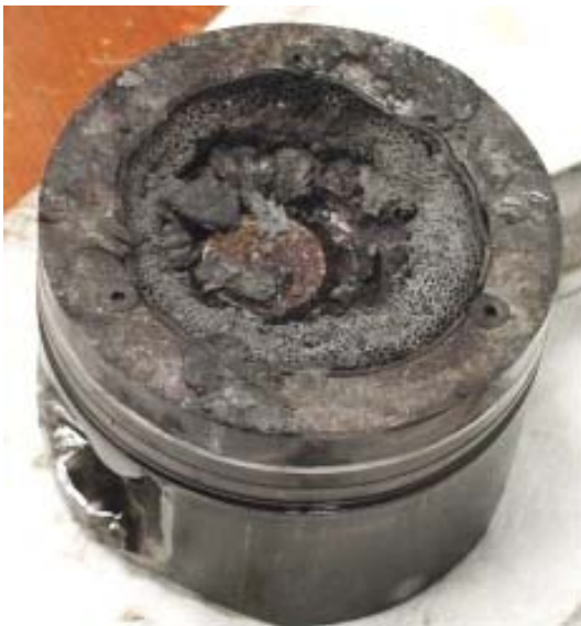
Figure 4. HCCI engine piston shown after catalyst failure.
