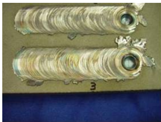
Figure 3 - Initial trials showing FSP can be used to stir thermal barrier coatings into steel plate. Surface coating was distributed into the substrate, but process parameter optimization and tool design changes will be needed to increase ceramic loading to the point where thermal conductivity is strongly affected.
