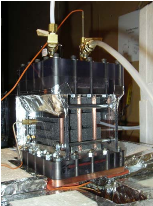
Figure 3. Instrumented thermal siphon with airside heat exchanger and boiling enhancements both made from high thermal conductivity graphite foam.
