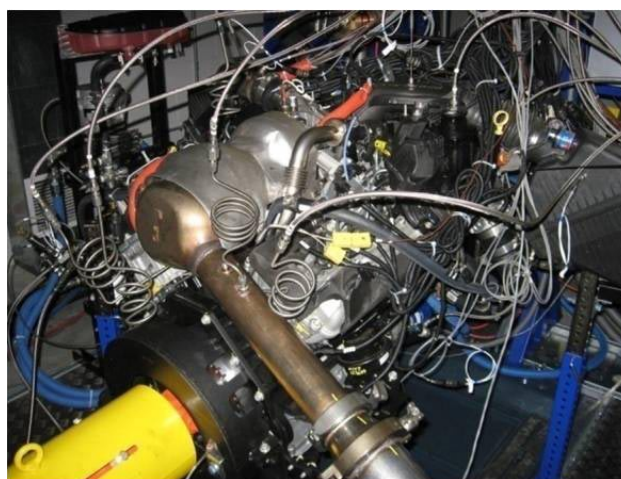
FIGURE 1. Multi-Cylinder Diesel Engine Installed in a Test Cell for Variable Valve Actuation Testing
