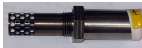
Typical EmiSense electronic soot sensor with electrode and shrouds on the left, M18 threads, and sensor body on the right. (Hall, UT at Austin)
