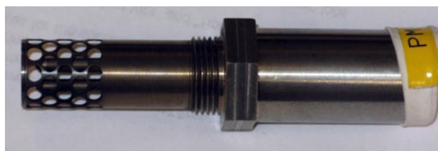
FIGURE 1. Typical EmiSense electronic soot sensor with electrode and shrouds on the left, M18 threads, and sensor body on the right.
