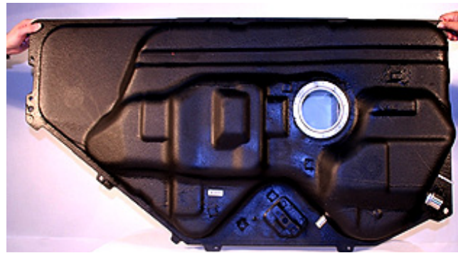
Figure 1. Photograph of one of the baseline sealed steel fuel tanks. Gross fuel tank mass 65 lbs/29.3 kg and 16 gallon capacity.
