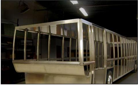
lighter than today's standard bus. An independent study performed by IBIS Associates, Inc., found that the new design achieves cost savings of 15–20% over the standard bus body.
