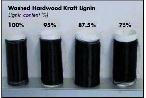
Lignin is a low-cost, renewable feedstock for carbon fibers.
