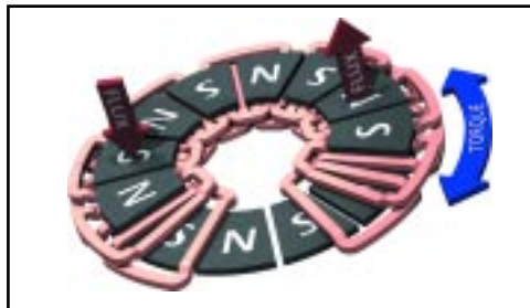
Patented SEMA coil design.
