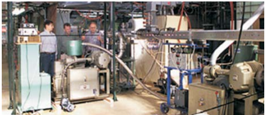
Researchers examine carbon fiber produced rapidly by the microwave/plasma processing device.
