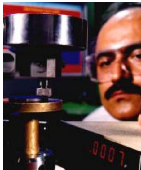
An Argonne researcher observes a sample of near-frictionless carbon (NFC) film that is 40 times slicker than Teflon™.
