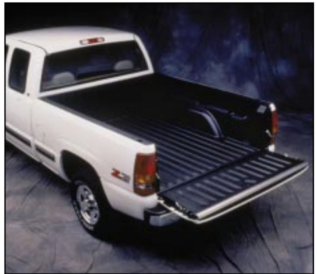
Composite truck bed installed in Chevrolet Silverado (photo courtesy of General Motors Corporation).
