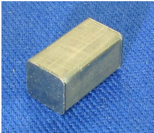
Metallized p-type \text{Yb}_{14}\text{MnSb}_{11} (Zintl) leg
