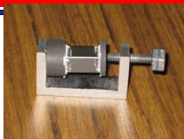
Coated Nano SiGe coupon coated after 9000 hrs of testing at 1273K
