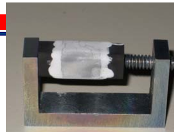
Coated Zintl coupon coated after 7000 hrs of testing at 1273K
