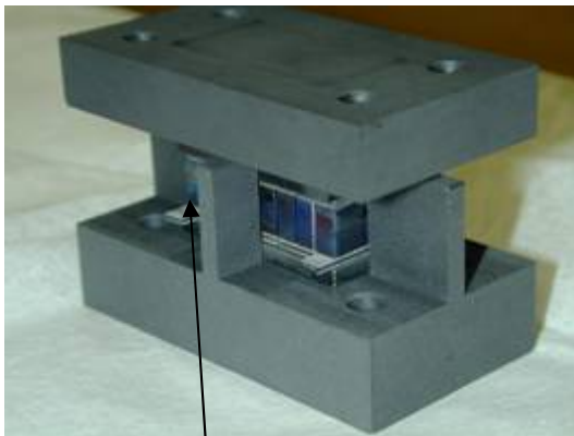
Assembled 2x4 Module after bonding cycle and egg-crate vaporized
