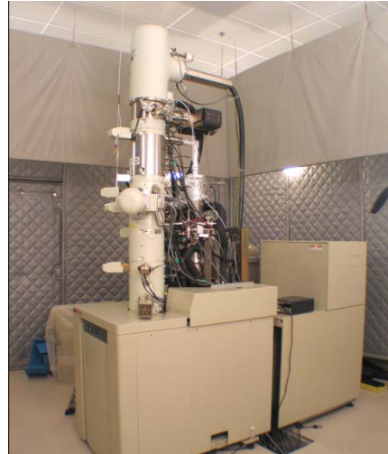
HTML's JEOL 2200FS STEM/TEM with aberration corrector for 0.7Å resolution in dark-field imaging
