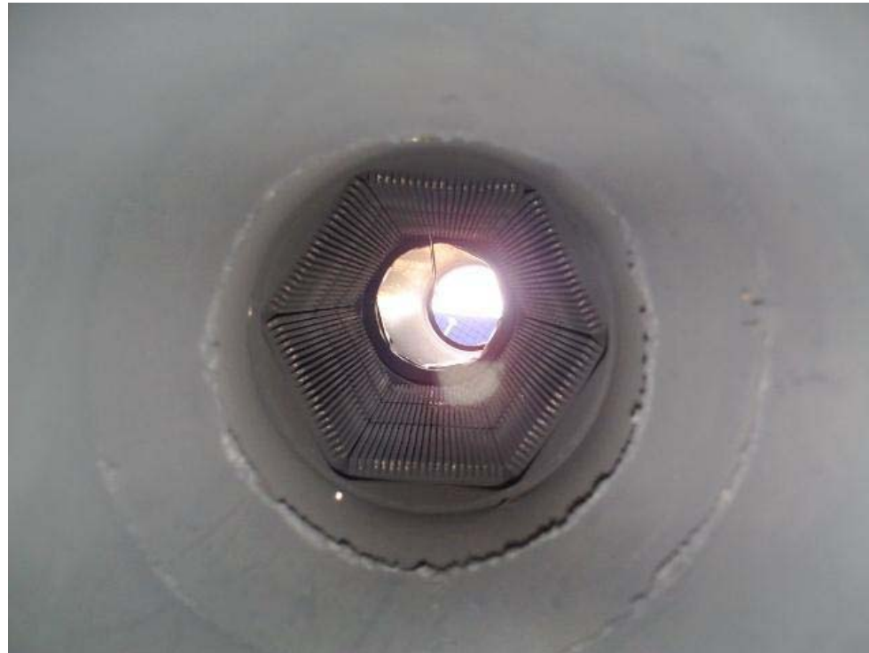
TEG Unit with Air Diffuser Removed
