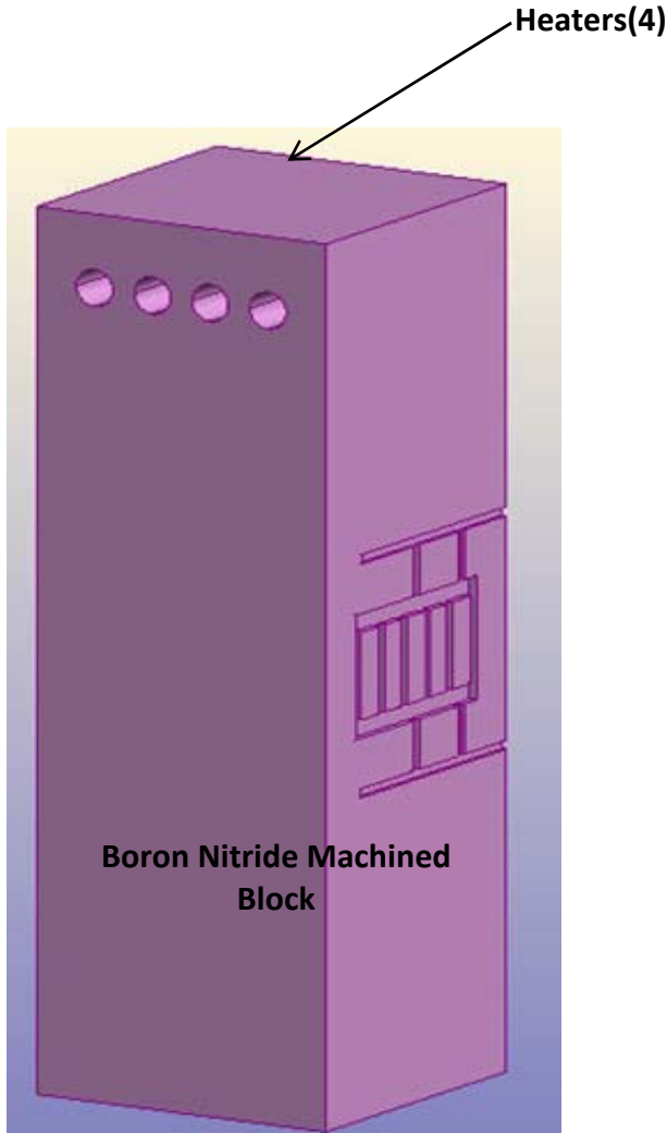
One Half of Boron Nitride Block showing three test pad locations
