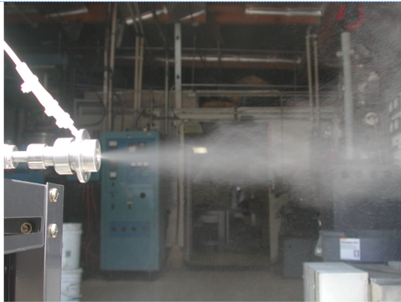
Aspirating Wick Atomizer Test. Fine Diesel Fuel Atomization
